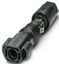
Photovoltaic connector, Range of articles: SUNCLIX, color: black, number of positions: 1, min. conductor cross-section: 2.5 mm<sup>2</sup>, max. conductor cross-section: 6 mm<sup>2</sup>, rated voltage: 1100 V DC, rated current: 35 A, Connection method: Spring-cage, min. cable diameter: 5.5 mm, max. cable diameter: 8 mm, Follow-up item to 1774687
